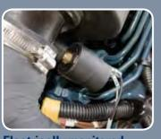
**Electrically monitored** air filter Air cleaner sensor alerts the operator of a restricted air filter and allows replacement before damage.
