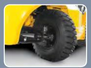
Fully hydrostatic power steering A hydraulic steering system always guarantees smooth and flexible steering, preventing overrun and kick-back.
