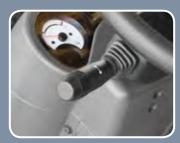
Easy and safe shift lever A single lever on the left side of the steering column gives the operator fast, easy control of direction.
